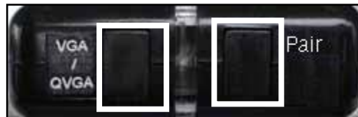
Figure 7.0 Press and hold the VGA/QVGA and Pair buttons at the same time
